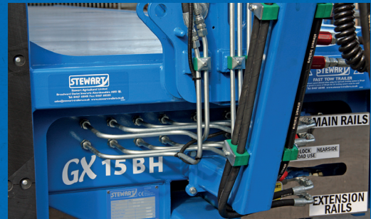
STAINLESS STEEL HYDRAULIC PIPES GIVE A TIDY FINISH
